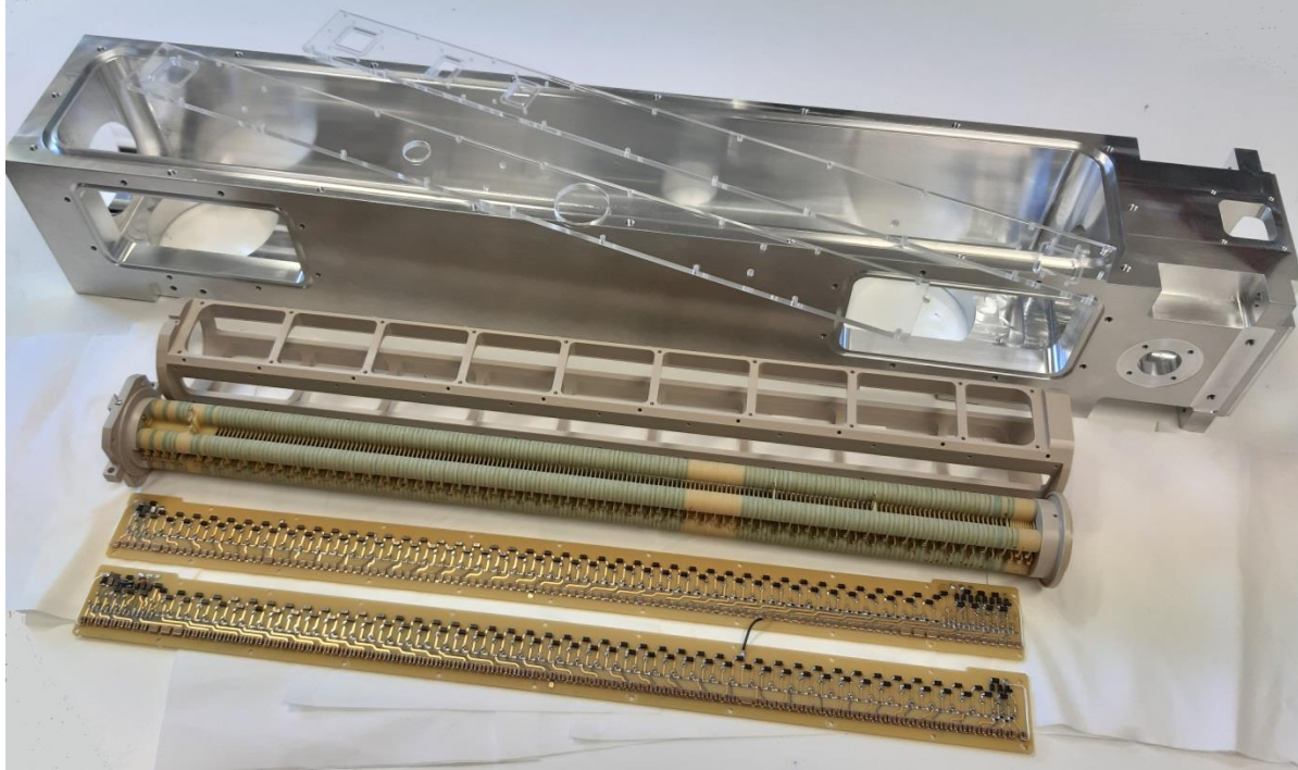
IMS outer & inner housing, drift pcb-electrode assembly, vacuum pcb's and electronics circuitries
