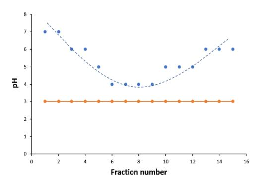
Plot: pH versus fractions eluted from the pl-trap cell without (blue) and with (orange) the buffer exchanger. An ampholyte with a pl range between 3-6 was used in these experiments.
