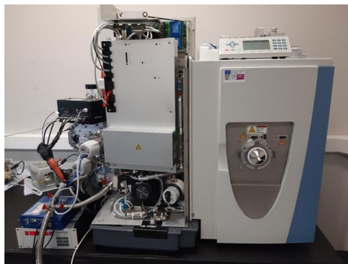
Figure 6.2. Q Exactive HF interfaced with the Omnitrap.
